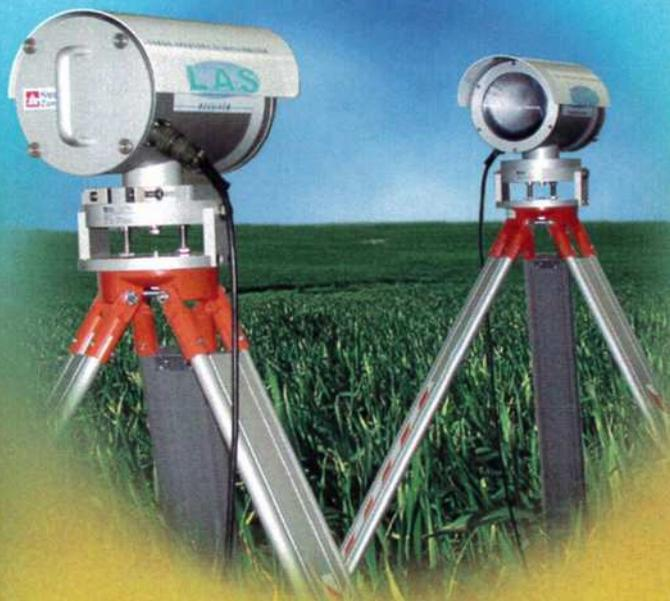
The line of sight path-integrating capabilities of the LAS (0.2 to 4.5 km) and X-LAS (1 to 10 km) provide reliable area-representative fluxes of sensible heat. The Scintillometers are also the basis of a complete system comprising selected environmental sensors, data loggers and specially developed software for the real-time measurement of evapo-transpiration, ideal for earth energy balance and water management studies.
