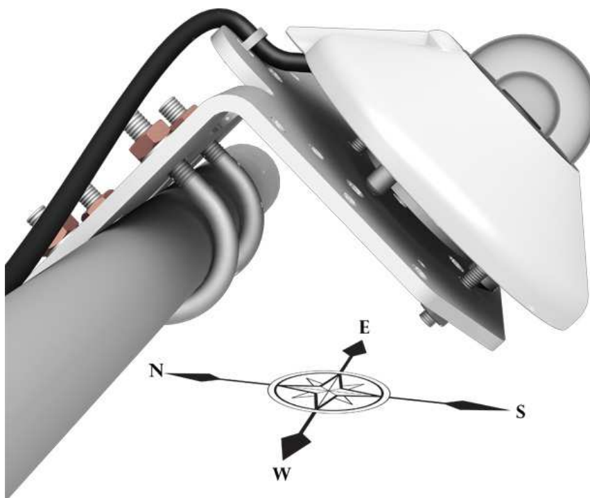
FIGURE 7-4. Pyranometer mounted at an angle for the Southern Hemisphere
