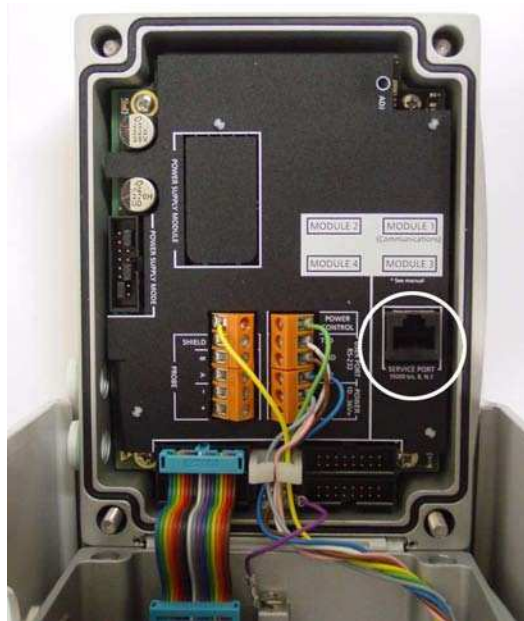
Figure 25 Service Port on the PTB330 Motherboard
