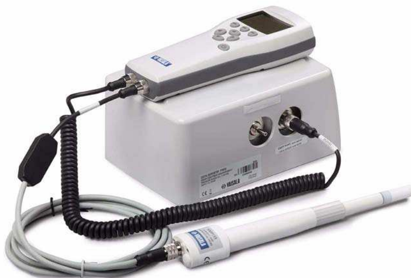
Figure 13 PTB330 and HMP155 Connected
